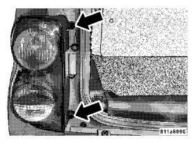
2. Rotate the light to the outboard side of the vehicle and remove.
